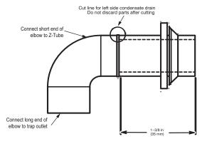
Fig. 17 - Modify Rubber Drain Elbow
