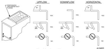
Fig. 20 – Duct Flanges
