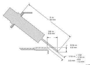
Fig. 68 – Igniter Position - Side View
