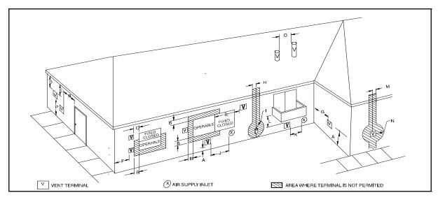
Fig. 47 – Ventilated Combustion Air and Non-Direct Vent Termination Clearance
