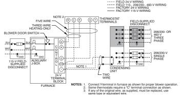
Fig. 32 – Typical Single-Stage Wiring Diagram
