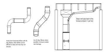
Fig. 51 – Near Furnace Vent Connections
