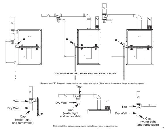
Fig. 50 – Recommended Combustion Air Inlet Moisture Trap
