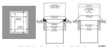
Fig. 25 – Installation on Combustible Flooring
