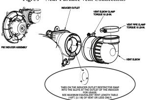
Fig. 52 – Inducer Vent Elbow
