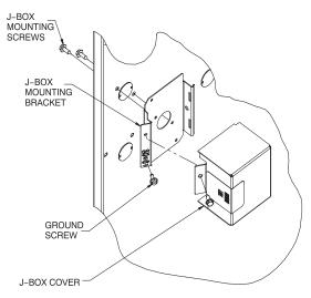
Fig. 34 – Installing J-Box (When Used)
