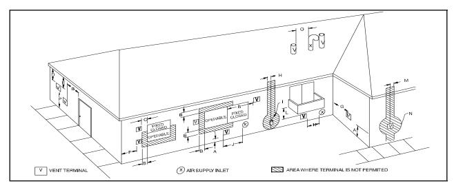
Fig. 46 – Direct Vent Termination Clearance
