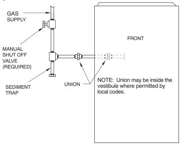
Fig. 31 – Typical Gas Pipe Arrangement
