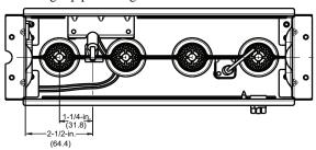
Fig. 67 – Igniter Position - Top View
