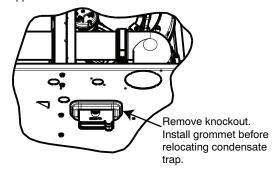
Fig. 18 – Horizontal Drain Trap Grommet
