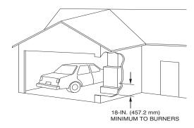
Fig. 5 - Installation in a Garage
