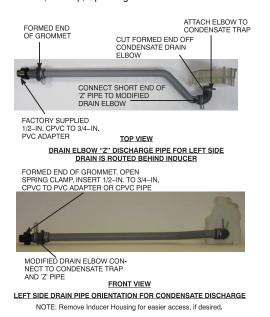
Fig. 16 – Drain Trap Connection and Routing (Appearance may vary)
