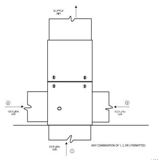
Fig. 21 – Upflow Return Air Configurations and Restrictions  $^{\rm A11036}$
