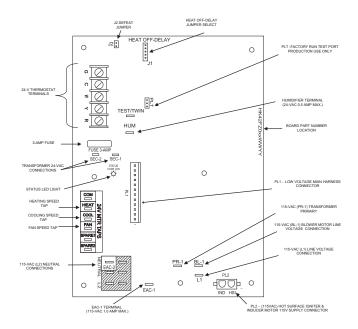
Fig. 36 – Example of Single Stage Furnace Control
