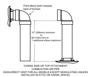
Fig. 43 – Combustion Air Pipe Attachment
