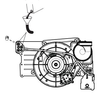
Fig. 59 – Priming Condensate Trap
