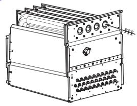
Fig. 69 – Cleaning Heat Exchanger Cell
