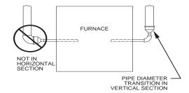
Fig. 49 – Combustion Air and Vent Pipe Diameter Transition A93034 Location and Elbow Configuration
