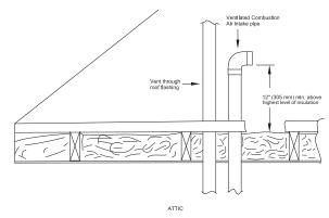
Fig. 45 – Vent Terminations for Ventilated Combustion Air  $^{\rm A10497}$
