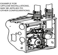
Fig. 41 – Sample Inlet Air Pipe Connection for Polypropylene A12220 Venting Systems
