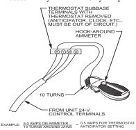
Fig. 64 - Amp. Draw Check with Ammeter
