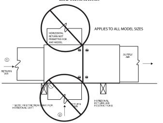
Fig. 23 – Horizontal Return Air Configurations and Restrictions
