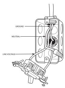
Fig. 35 – Field-Supplied External Electrical Box on Furnace Casing
